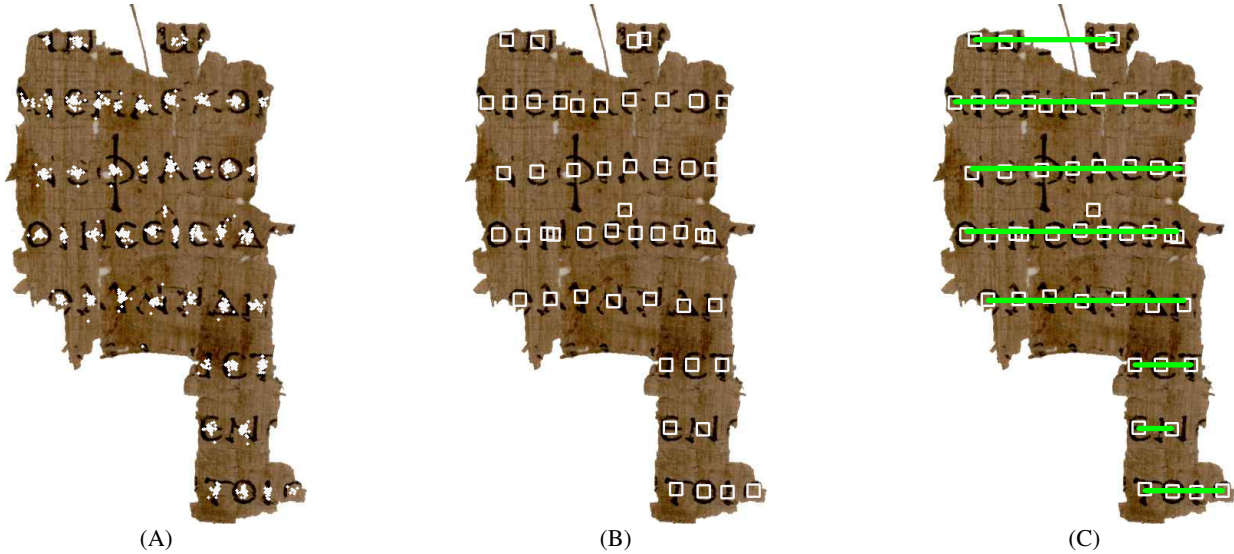
Fig. 3: A visualization of the processing performed by the pipeline using the same Ancient Lives fragment from Figure 2. A) White dots represent the 1,591 clicks of all users. B) White squares represent calculated consensus clicks from the aggregated click data of all users for the fragment using the stepwise aggregation approach. C) Green lines represent the regression line for the nearby consensus clicks.
